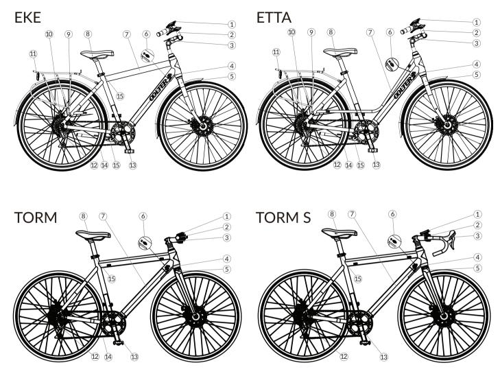
1. Display6. Main switch2. Handlebar7. Frame3. Stem8. Seat4. Charging port9. Luggage rack5. Front Fork10. Motor
