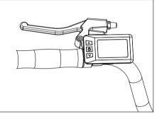
For activating the display, press and hold the power button until the display lights up. Do the same again to deactivate the display. Display auto-off happens after 5 minutes idle.
