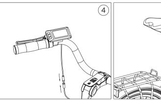
Attach the reflector and bell to the handlebar. The display is installed on the left side of the handlebar. Adjust it to the position pictured on diagram 4. Fasten the display to the handlebar using the M3 screw on the underside of the display and connect the display cable.
