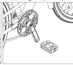
Install the left (L) and right (R chain-side) pedals by turning them by hand first. Tighten with a 15mm wrench with no excess force (150Nm). Note that the pedals for the left and right side have different thread and cannot be mixed.
